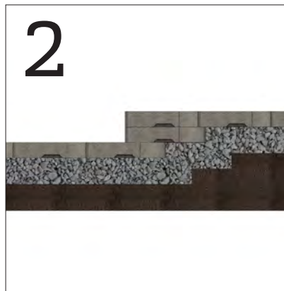
Install Base Course
